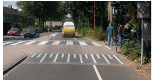
Crossing (raised section, marking)
