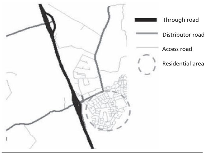
Figure 1.5. Three functional road types as the basis of sustainably safe road traffic [1.64]
