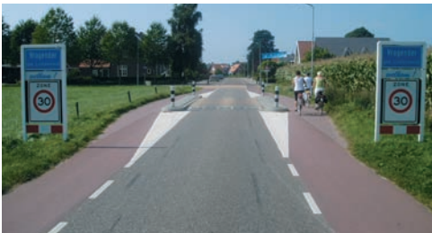
Area boundary on access road, raised road section and bicycle paths
